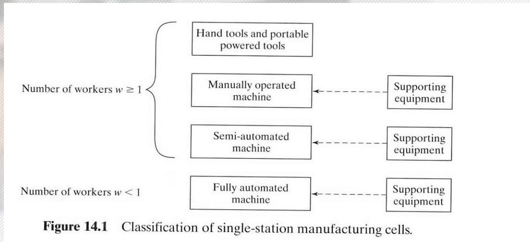
Fuente: Mikel P. Groover. Automation Production System And Computer Integrated Manufacturing.
